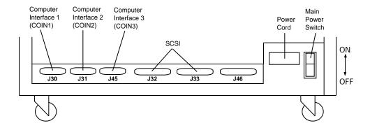
Computer Interface 1 (COIN1) - Service/Diagnostic Interface. Used when configuring the Scanner and for running diagnostics.
